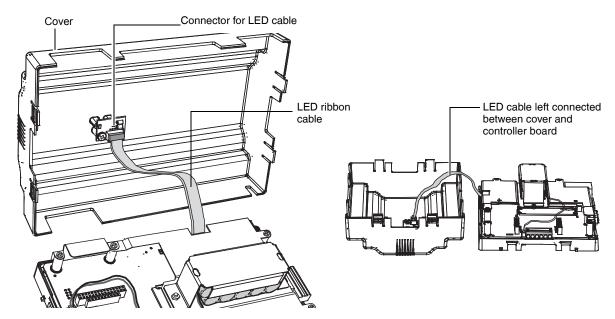
Fig. 4. Removing WEB/CP-700 cover.
